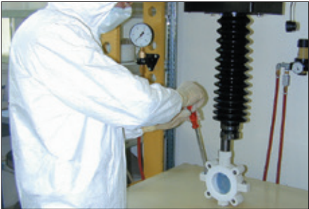
Valve assembly in clean room
