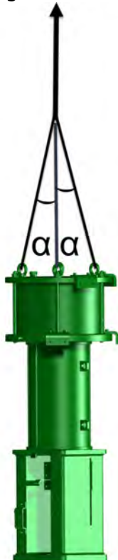
Figure 9. Lifting Angle for Welded Eyelets
