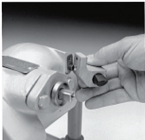
Step 8 Place latch block on body with lower blind hole over bolt in body.
