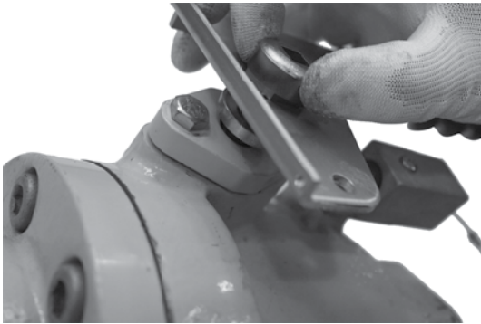
Figure 23. Install handle (step 12)
