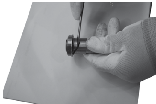
Figure 6. Remove O-ring (step 7)
