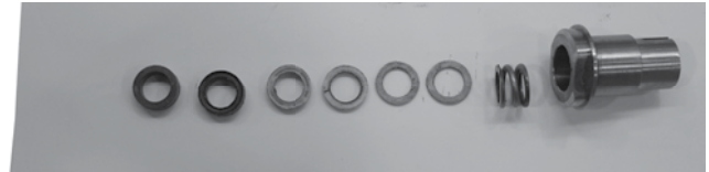
Figure 8. Remove packing carefully (step 8)
