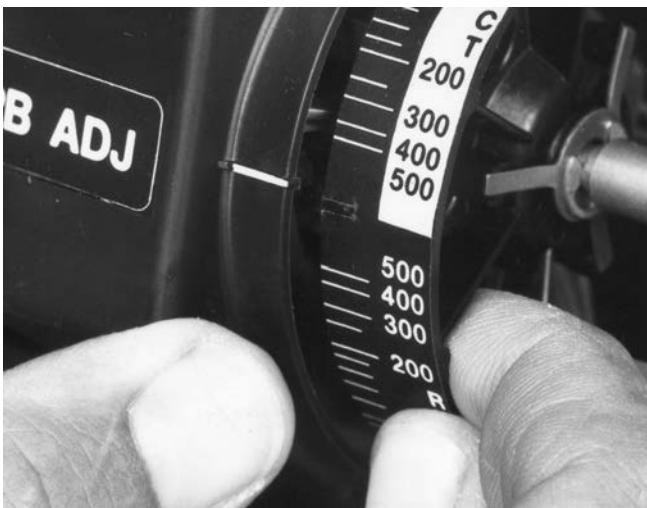
Figure 24. Changing Controller Action (Fisher 4196S Controllers)
