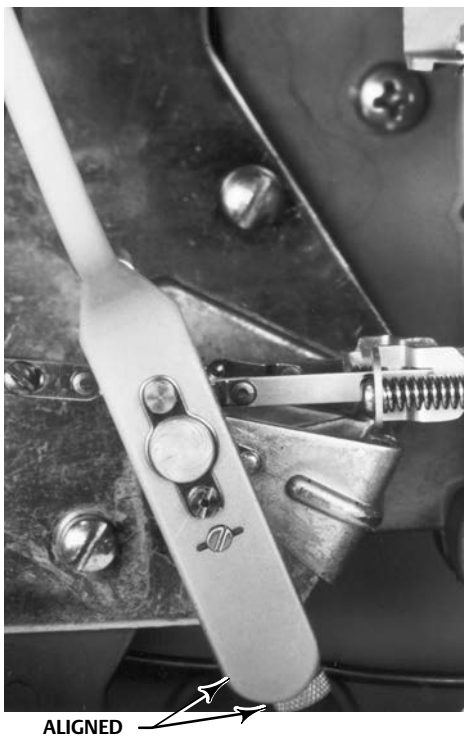
Figure 42. Process Pointer Alignment
