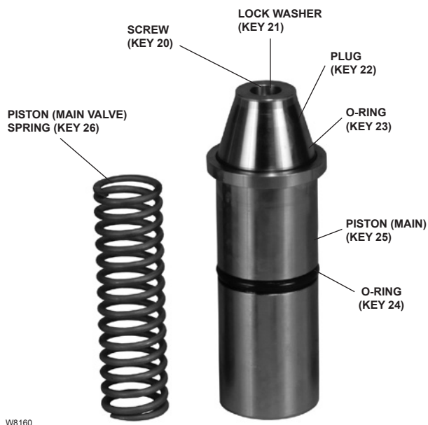
Figure 10. NPS 2 / DN 50 Pad Valve Piston and Spring
