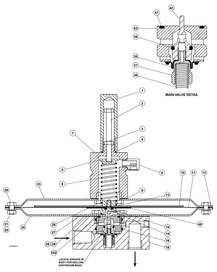
Figure 6. Type ACE95jr Tank Blanketing Valve Assembly
