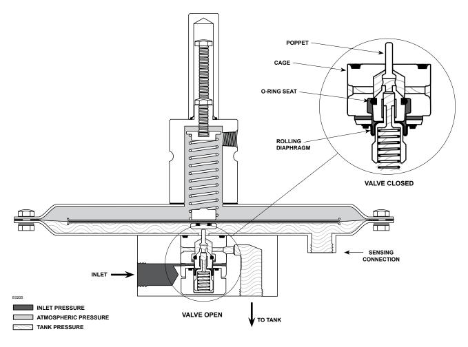
Figure 2. Type ACE95jr Operational Schematic
