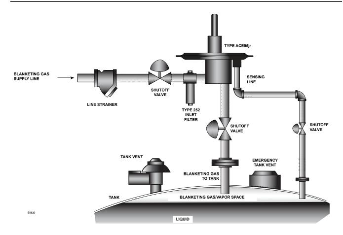
Figure 3. Type ACE95jr Tank Blanketing Valve Installation
